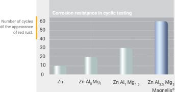
10 µm of coating submitted for an alternated cycling of 8 hours fog cycle (5% NaCl) / dry cycle / humidity cycle.
